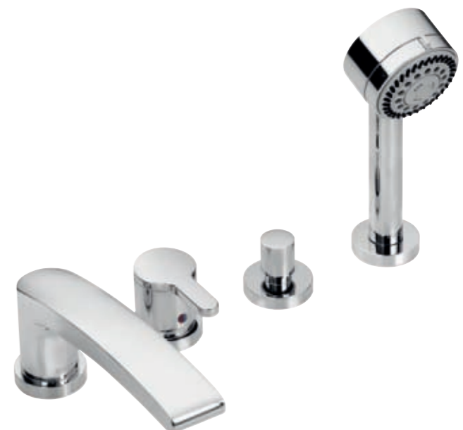
51630 Single lever bath tub and shower mixer 4-hole bath deck-mounted, cartridge mixer with ceramic sealing gaskets, with automatic return bath tub/shower, concealable hand shower with normal-, soft-, and massage jet
