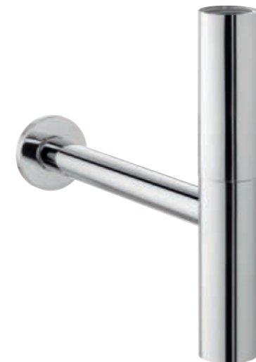
59906 Design bottle trap G 1 1/4 inch, telescopic inlet tube 140 mm, wall tube 330 mm, rosette Ø 72 mm
