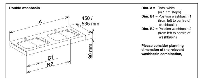
Lateral veneer through side panels or base cabinet module. For the planning of the washbasin board please consider the lateral veneers: A) Washbasin board without/with base cabinet module If an right
