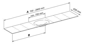
**Dimension A** = total width (700 - 2800 mm, in 350 mm steps) **Dimension B** = position of the wash basin bow (from left to centre of basin, in 350/175 mm increments)
